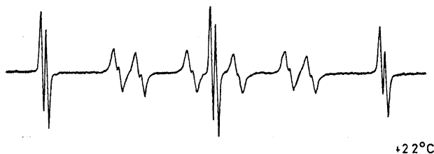
Fig. 3. ESR spectrum of the radical \text{H}-\overset{\ominus}{\text{C}}(\text{NO}_2)_2^- .
